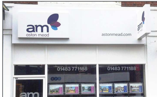
Internally illuminated, built up aluminium sign tray. Fret cut logo and backed up with an acrylic sheet. Supplied with an illuminated projecting sign.
