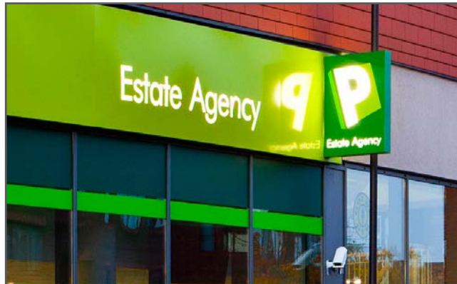
Internally illuminated, fret cut aluminium projecting sign, fixed flush to the fascia sign.
