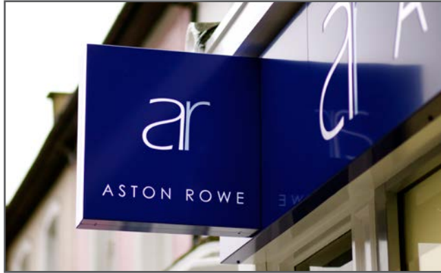
Fret cut, internally illuminated using LED lighting and fixed to the wall with powder coated brackets.
