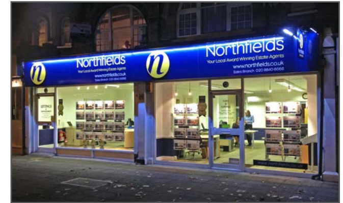
Aluminium sign tray with 10mm acrylic stand off logo and company name with vinyl text. LED parabeam and an illuminated projecting sign.
