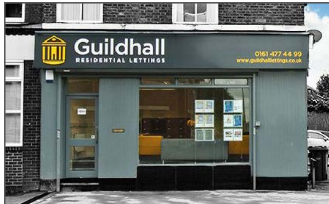
Dibond corner sign tray, with stand off lettering and illuminated via an LED parabeam
