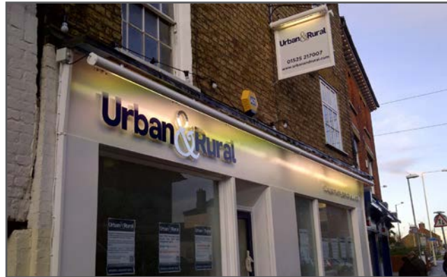
Stand off dibond lettering direct to fascia board, illuminated with a parabeam. Supplied with an illuminated hanging projecting sign.
