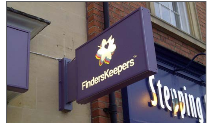
Internally LED illuminated with all text fret cut. Individual letters faced with vinyl to create a halo effect.
