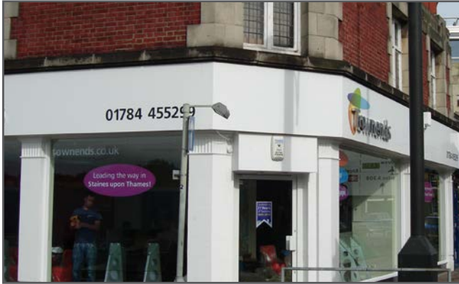
Shaped, fret cut and internally illuminated. Fixed through sign tray using a 'top hat' bracket.
