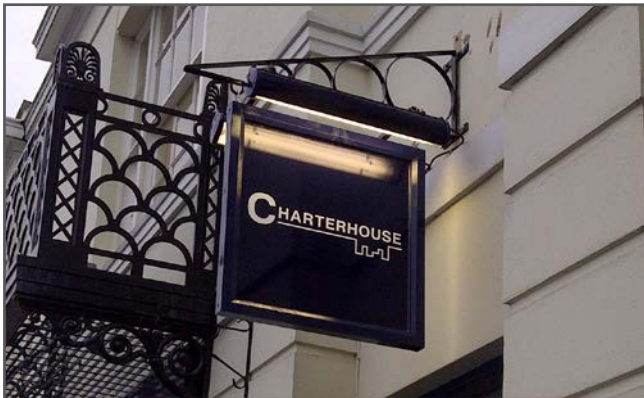
Traditional projecting sign on wrought iron bracket with mini parabeam lights using LED illumination.
