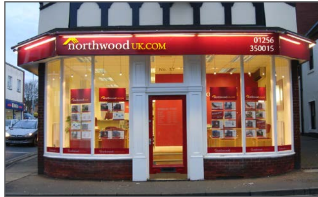
Aluminium sign tray with mitred corners, 5mm acrylic stand off logo and company name, fluorescent parabeam and an illuminated projecting sign.
