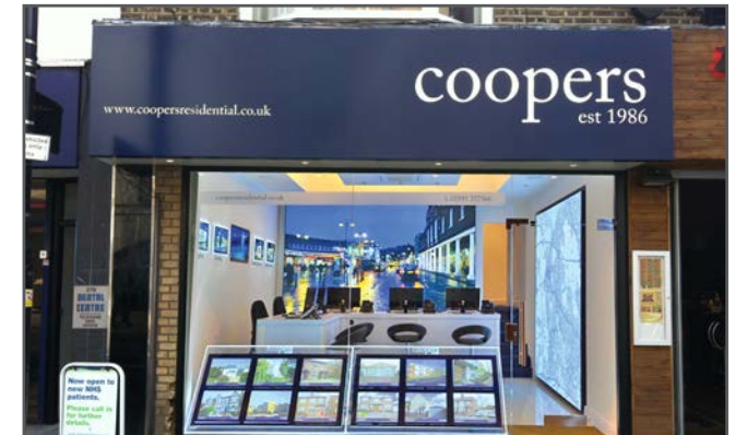
LED illuminated flex face fascia with powder coated back tray. Tensioned, digitally printed PVC allowing full illumination across the whole sign.
