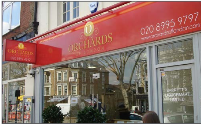
Aluminium sign tray with 5mm acrylic text bonded direct to face of sign. Colour coded fluorescent parabeam and internally illuminated projecting sign.
